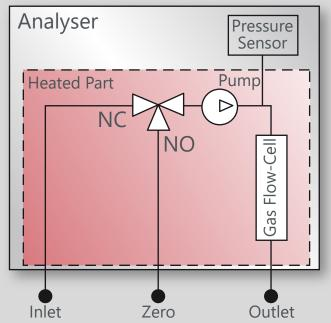
Inlet and zero are connected on a 3 ways electric valve. When the automatic zero is activated, the solenoid valve switches the flow cell on zero air. A pressure sensor takes the pressure of measured gas to compensate it and to give a flow indication.
