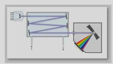
The measuring principle is based on the UV light absorption according to the Beer-Lambert Law:
